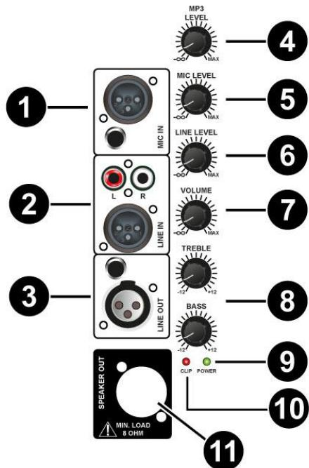
1. Input connector for microphone.
