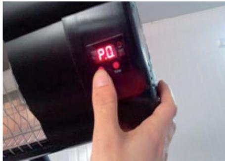
3. Press Open/Close second, the digital screen shows P.1, means low heating (850 W).
