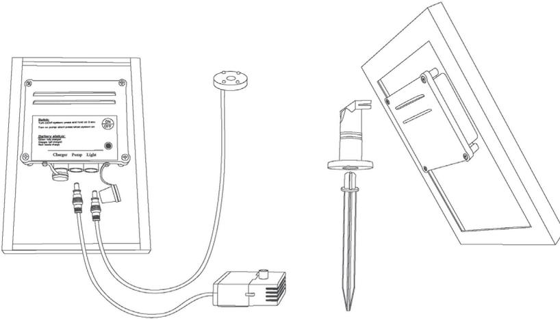
This solar pump is designed primarily to operate in sunlight hours and always charge extra energy to battery to allow use later "on demand" in cloudy day or night time. The pump will turn to solar mode automatically on next day in sunlight hours. The pump will never run on battery mode until your press the button.
