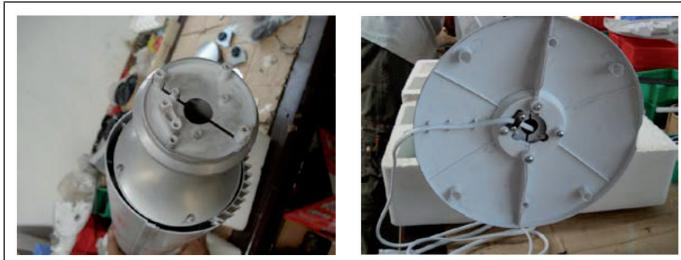
3. Place the fan on the base and fix it by tightening the 3 long screws with the screwdriver.
