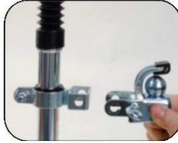
Secure the saddle-support mounting with the help of the plastic shims to the seat post of your bicycle.
