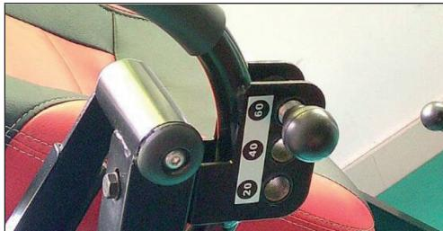
Familiarise yourself with the quick adjuster on the right-hand side. The position of the locking pin determines the inversion angle you are comfortable with. The 3 settings are:
