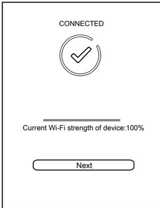
8. After connected, the following screen will appear. Tap "Custom..." to set a new desired location name, or tap one in the name list as the selected location.
