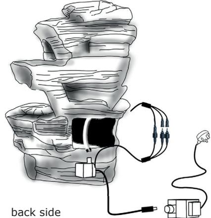
4. Connect the pump to the adapter and plug in.
