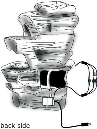
3. Connect the 3 wires for the LED lights.
