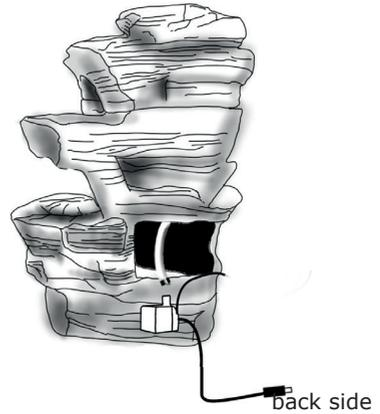
2. Pull out the tube and connect it to the pump.
