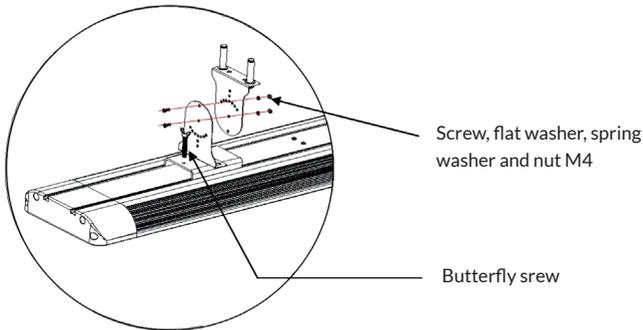
Connect the two adjustment brackets and tighten the sliding bracket with the butterfly screw.
