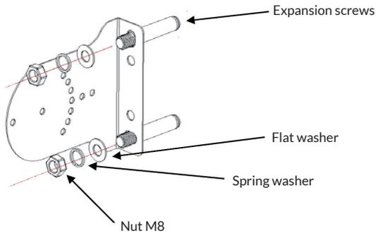
Attach the adjustment brackets to the wall.
