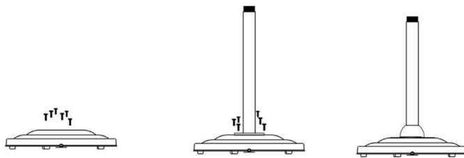
Remove 6 pcs M6\*30 mm screws in base, fix bottom tube to the base and put the decorative cover into it.
