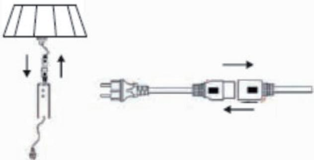
Fix the heater head to the top tube and connect the power cord together and fix by the plastic cover.
