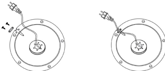
Fix the power cord to the base by 2 pcs ST6\*14 mm screws.
