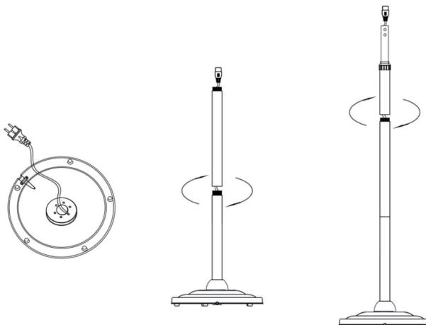
Through the power cord to middle and top tube and screw all tubes together.
