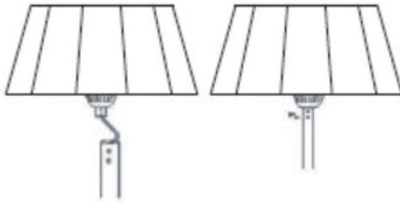
Fix the heater head to top tube by 2 pcs ST4\*10 mm screws.
