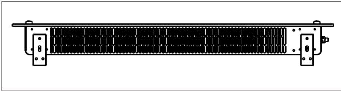
3. Hold the side of the product, look at the position of the wall hole of the rear cover, and slide the wall to the top of the slot, that is, the installation of the wall is completed, as depicted in the picture below.
