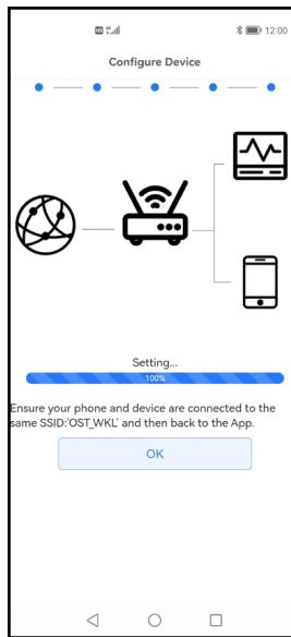
Connect the **EasyWeather-WIFI** weather station to your router via your mobile device. If the connection was established successfully, the upload settings will be displayed automatically.
