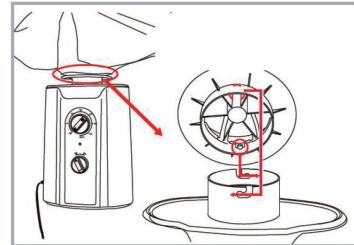
Open the zip of air bag, and put the cover on to motor, install the outlet vent on the motor.
