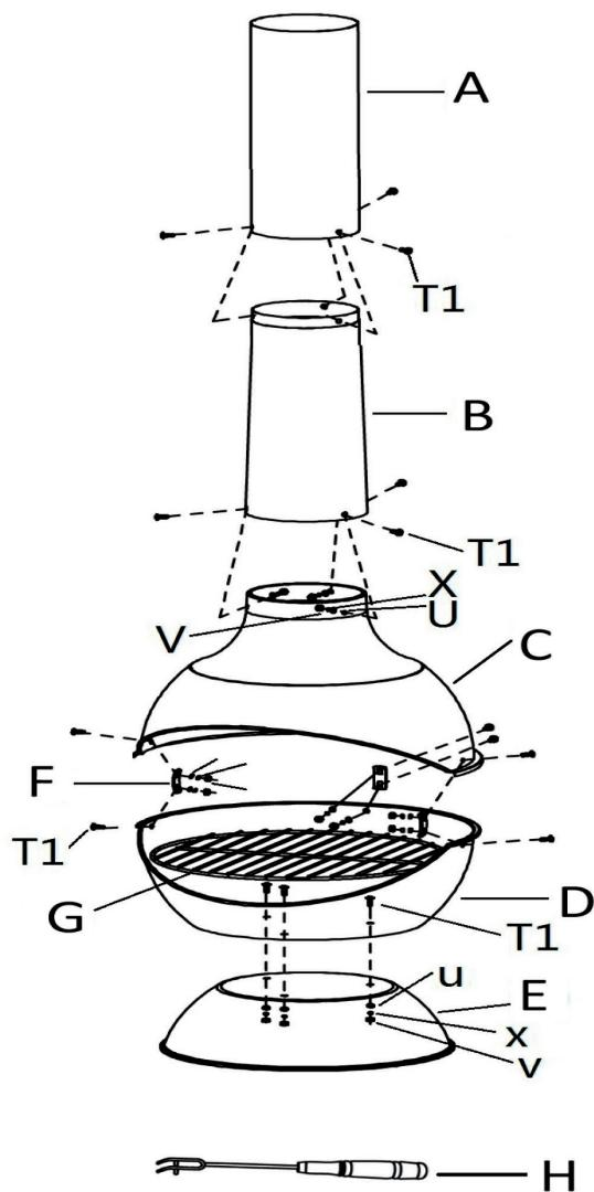
**Note:** do not fully tighten the bolts before assembling all the parts. Assembly is easier with two people, one to hold the parts and a second person to insert the fixings.
