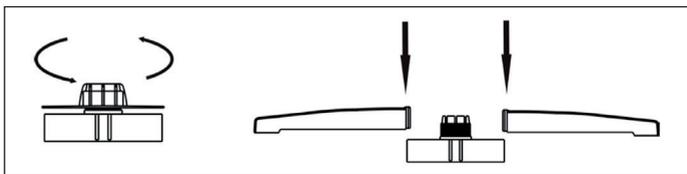
2. Fix the stand to the base by using the base cover as below.
