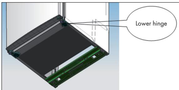
6. Replace the bottom door bearing bush and the limit block.
