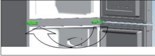
9. Place the upper door on the middle hinge and then attach the upper suspension. Finally, fasten the screw caps and replace the covers. Level out small unevenness in the floor with the adjustable feet.
