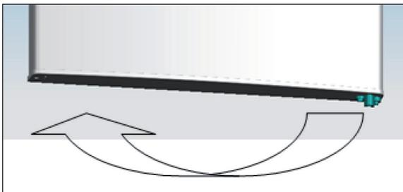
7. Replace the bottom hinge to the other side then fix it with screws.
