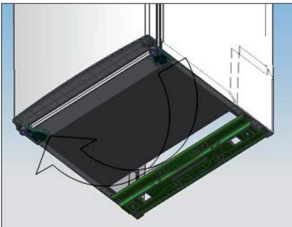
8. Place the lower door on the lower hinge. Then attach the middle hinge to the opposite side.
