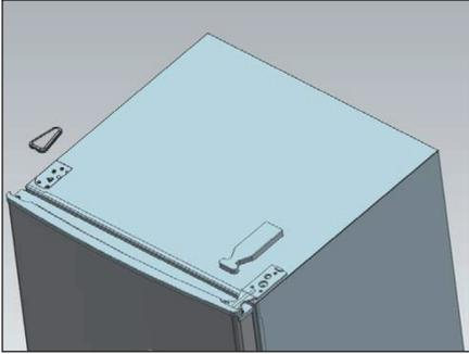
2. Replace the top-hinge and the top-door limit block and the door bearing bush to the other side. Remove the nut with sleeve. Take off the washer then remove the axes to the other side and fixed.
