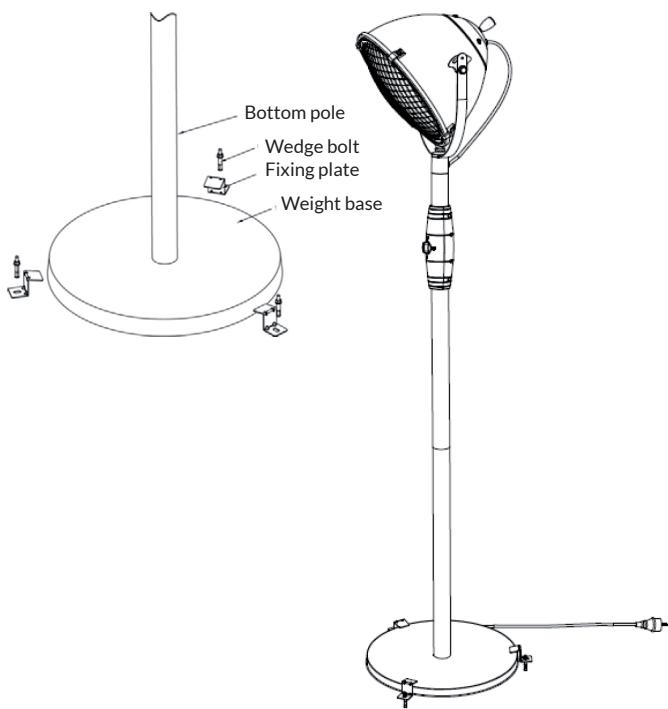
Fix the heater on the floor. Bore three holes in the floor, fix the heater by three wedge bolts on the floor tightening the screws by spanner.
