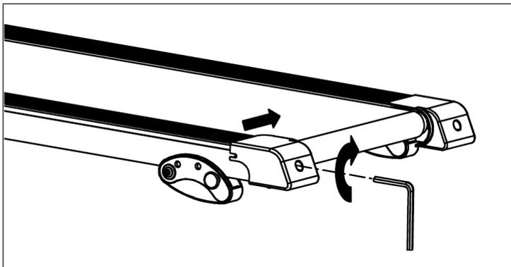
If the running belt is shifting to the left, turn the left adjustment bolt 1/4 turn clockwise, and the running belt should start to correct itself.
