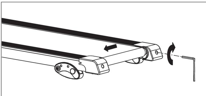
If the running belt is shifting to the right, then turn the right adjustment bolt 1/4 turn clockwise, and the belt should start to correct itself. Keep turning the adjustment bolts until the running belt is properly centered.
