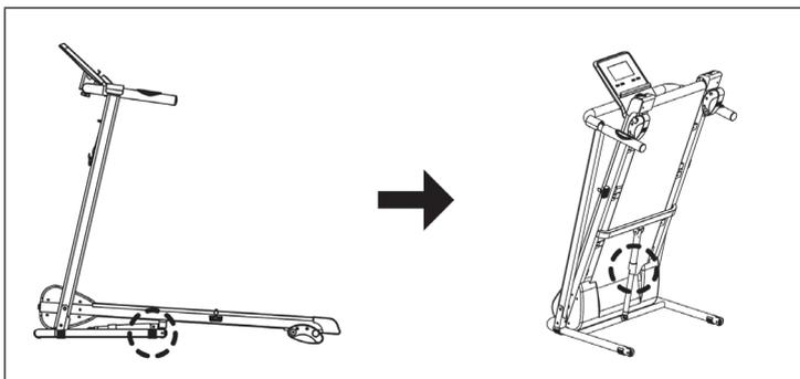
After use, unscrew the safety lock on the bottom frame, fold the treadmill and pull the expandable safety lock out from the left Upright and release to lock the treadmill in an upright position. To avoid losing the safety lock, screw the safety lock to the bottom and upper frames whilst in an upright position.
