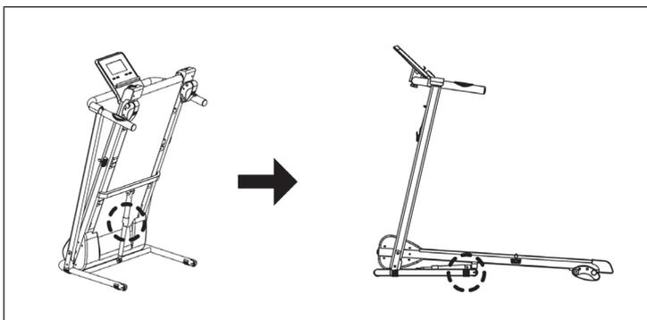
Unscrew the safety lock on the bottom frame, release the expandable safety lock and lower the bottom frame to the ground. Screw the safety lock to the bottom frame to lock the upper frame in an upright position.
