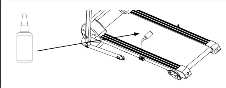
Lift one side of running belt. Pour some lubricant under the centre of the running belt on the top surface of the running deck. Run on the treadmill at a slow speed for 3 to 5 minutes to evenly distribute lubricant.
