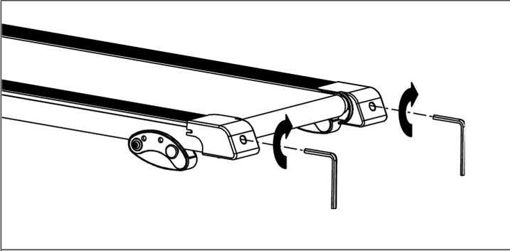
If the running belt is slipping during use, turn off and unplug the treadmill. Using the 6 mm Allen Wrench provided, turn both left and right rear roller adjustment bolts 1/4 turn clockwise, then turn the main power switch back on and run the treadmill at a speed of 8-10 KPH. Run on to the running belt to determine if the belt is still slipping. Repeat this procedure until the belt no longer slips.
