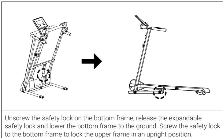
Unscrew the safety lock on the bottom frame, release the expandable safety lock and lower the bottom frame to the ground. Screw the safety lock to the bottom frame to lock the upper frame in an upright position.
