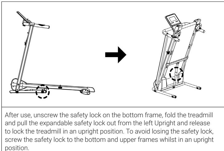
After use, unscrew the safety lock on the bottom frame, fold the treadmill and pull the expandable safety lock out from the left Upright and release to lock the treadmill in an upright position. To avoid losing the safety lock, screw the safety lock to the bottom and upper frames whilst in an upright position.
