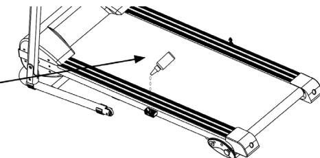
Lift one side of running belt. Pour some lubricant under the centre of the running belt on the top surface of the running deck. Run on the treadmill at a slow speed for 3 to 5 minutes to evenly distribute lubricant.
