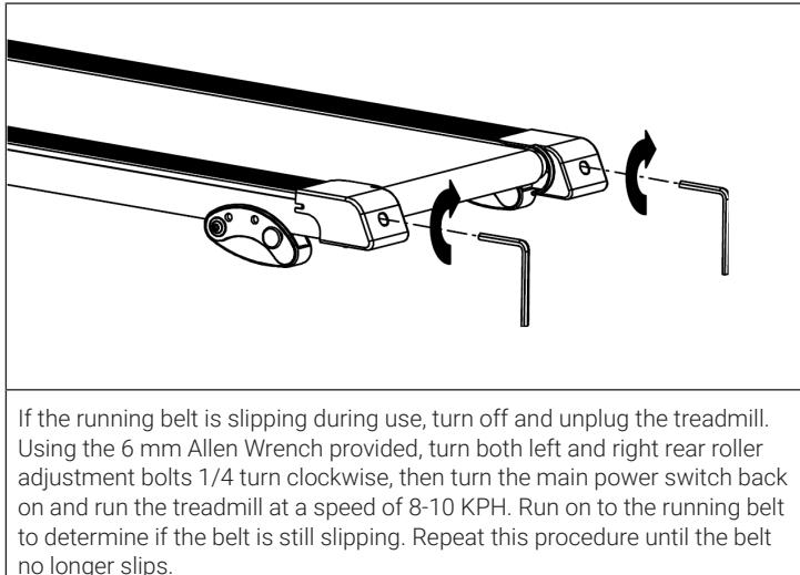
If the running belt is slipping during use, turn off and unplug the treadmill. Using the 6 mm Allen Wrench provided, turn both left and right rear roller adjustment bolts 1/4 turn clockwise, then turn the main power switch back on and run the treadmill at a speed of 8-10 KPH. Run on to the running belt to determine if the belt is still slipping. Repeat this procedure until the belt no longer slips.
