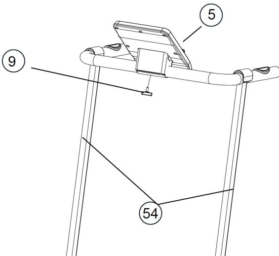
A. Turn the Computer Console (5) up or down to align the Socket Head Screw hole.
