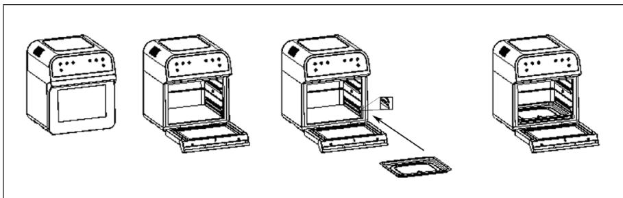
Carefully open the door and slide the drip tray into the unit on the side rails as shown in the picture.
