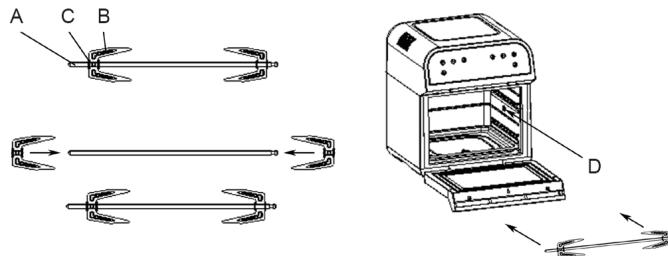
Slide the fixators (B) onto the rotisserie rod (A). Tighten the screws of the fixators (C) so that the fixators are firmly attached to the rotisserie. Insert the rotisserie into the rotators (D) in the appliance. It only fits in the rotators a certain way. Do not use force.
