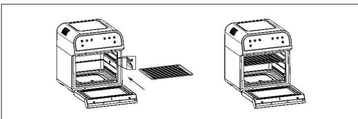
Carefully open the door and slide the drip tray into the unit on the side rails as shown in the picture.
