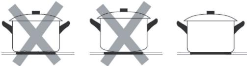
Cookware made from the following materials is not suitable: pure stainless steel, aluminium or copper without a magnetic base, glass, wood, porcelain, ceramic, and earthenware. Do not use cookware with jagged edges or a curved base.
