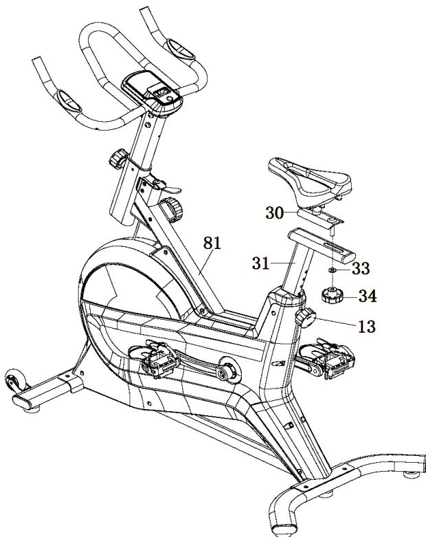
Attach the Seat Slider (No.30) to the Seat Post (No.31), tighten and secure with Washer (33) and Knob (No.34).
