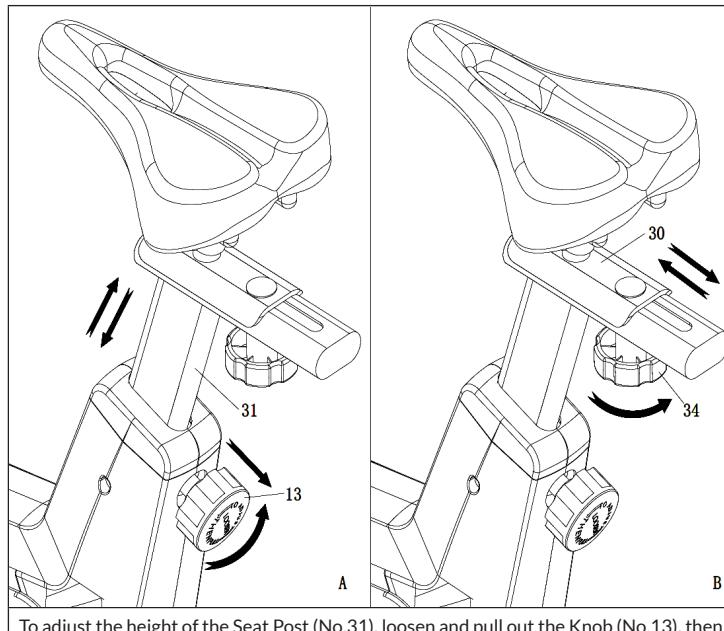
To adjust the height of the Seat Post (No.31), loosen and pull out the Knob (No.13), then raise or lower the seat to the desired height. Once adjusted, re-insert and tighten the Knob (No.13) to secure the seat in place. (Figure A)
