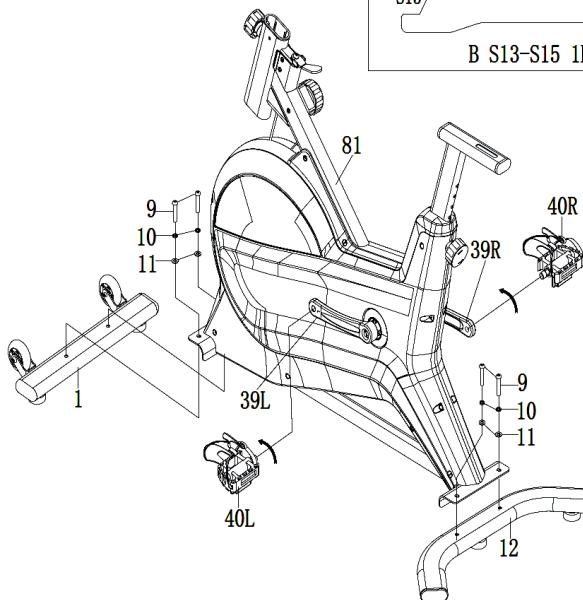
Attach the Front & Rear Stabilizer (No.1 & 12) to the Main Frame (No.81) using 4 Screws (No.9), 4 Spring washers (No.10) and 4 Washer (No.11). Tighten with an Allen Wrench (No.A).
