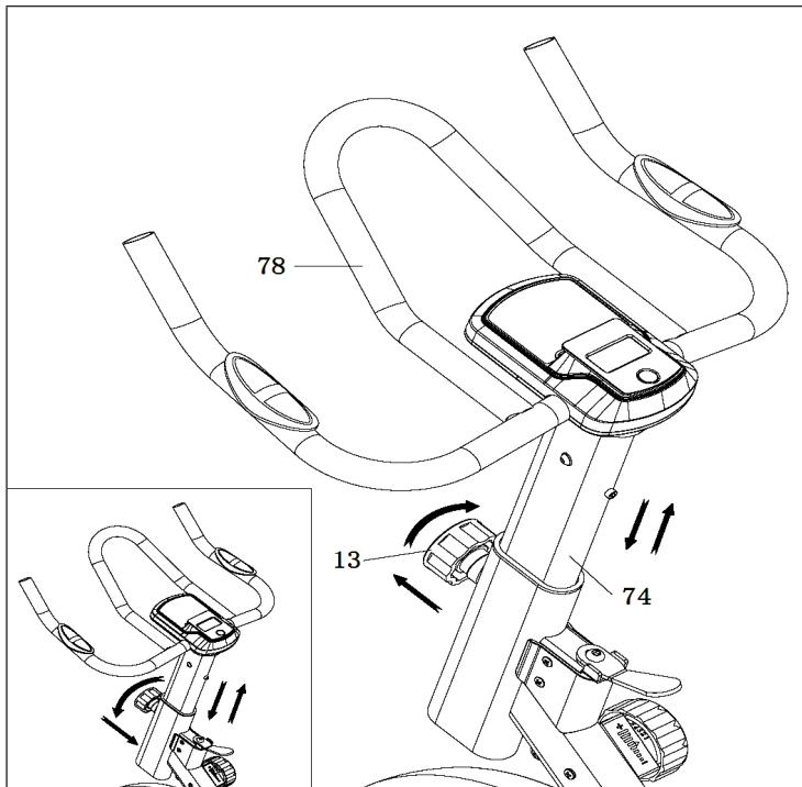
To adjust the height of Handlebar (No.78), loosen and pull on the Knob (No.13), then slide the Handlebar Post (No.74) up or down to the desired height. Once adjusted, tighten the Knob (No.13) to secure the Handlebar Post (No.74) in place.
