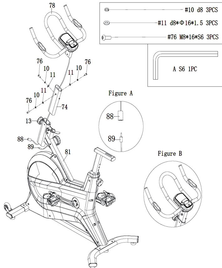
Insert Trunk line (No. 88) through Seat Post (No.74). Then attach the Handlebar (No.78) to Handlebar Post (No.74) using 3 Screws (No. 76), 3 Spring washers (No. 10), and 3 washers (No. 11). Tighten with an Allen Wrench (No.A). (Figure B)
