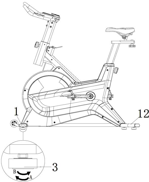
To achieve a smooth and comfortable experience, you must ensure that the bike is stable. During use, if you notice that the bike is unbalanced, you can adjust the Foot Pads (No.3) located beneath the Front & Rear Stabilizers (No.1 & 12).
