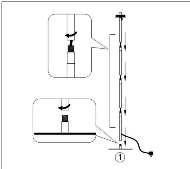
1. Put the wire through the four segments. Connect the four segments together by turning them clockwise and attach them to the lamp base.
