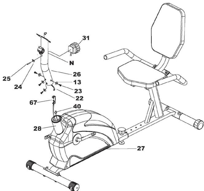
A) Take the Front Post (26) and join the Middle Computer Wire (22) with Lower Computer Wire (40). Pull Lower Tension Cable (67) from Front post (26) and out from the hole on the upside, then connect the Lower Tension Cable (67) with Tension Cable (31), like the arrow direction. Then fasten the Tension Knob by 1x Curve Washer (24) & Screw (25).
