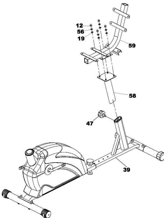
A) Insert the Seat post (58) into the Rear main frame (39), then tighten with Spring knob (47).
