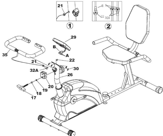
A) Fix the Handlebar (35) to the Front Post (26) and tighten with 1x Cover of handlebar(20), 1x Washer (19), 1x Spacer (18) and 1 x T Knob (17). Get the Middle pulse wire (32A) through the powder A (21) , pull up from the middle of Front Post (26).
