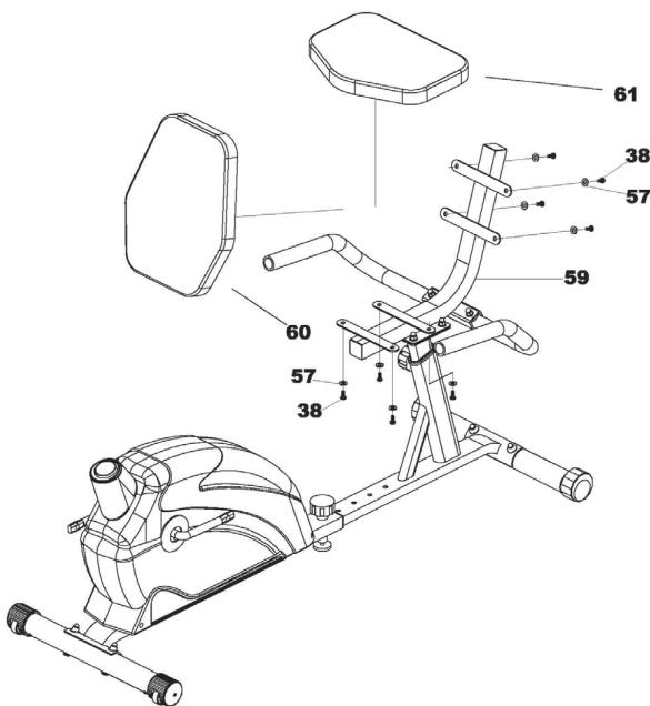
A) Attach the Seat (61) to the Back cushion tube (59), using 4x Flat Washer (57) and 4x Allen bolt (38).
