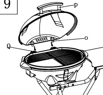
Mount the cover. Hold the cover by the handle (p) and slide the hinges (O) into the holes (Q) of the base. When you later remove the cover, open the cover at a 45° angle and release the hinges (O) from the holes (Q). The cover must be open at a 45° angle for it to be removed.
