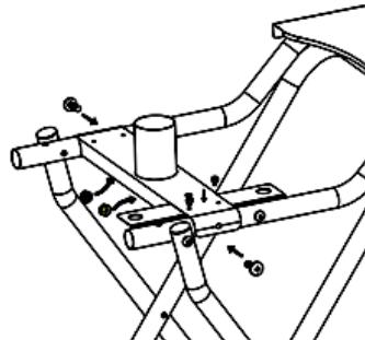
First remove the screw from the pipe. Mount the bracket (G1) on the pipe. Then mount the support tube (G2) on the tube. There is a positioning hole (IV) on the support tube (G2) where the housing is later fixed. Tighten the bracket (G1) and the support tube (G2) with screws and nuts.
