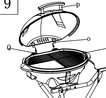
Mount the cover. Hold the cover by the handle (p) and slide the hinges (O) into the holes (Q) of the base. When you later remove the cover, open the cover at a 45° angle and release the hinges (O) from the holes (Q). The cover must be open at a 45° angle for it to be removed.
