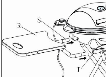
Mount the table (R). Hold the table (R) firmly and press down the two pins (S) with your thumbs. Then insert into the tube (T). Later, remove the table (R) before folding the trolley. Press down the pins (S) and carefully pull out the tube (T).
