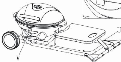
If you move the collapsed trolley or if the unit is not in use, lock the cover with the buckle (W) located on the housing. Make sure that the latch (V) is tight.
