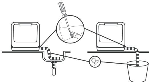
Insert the end of the drain hose into a sink or bucket. Fix the drain hose with suction cups.
