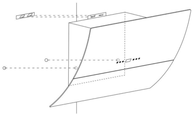
For inclined panel model, you need to drill 2 x 8 mm extra holes and use screw plugs and screws before installation.
