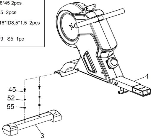
Attach the front stabilizer tube (#3) to the main frame (#1) using 2 washers (#55), 2 spring washers (#52) and 2 Allen screws (#45).
