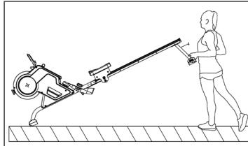
To move the machine, lift up the rear stabilizer until the transportation wheels on the front stand touch the ground. With the wheels on the ground, you can transport the rower to the desired location with ease.
