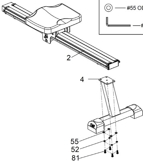
Attach the rear support tube (#4) to the slide rail (#2) and tighten with 4 washers (#55), 4 spring washers (#52) and 4 Allen screws (#81).
