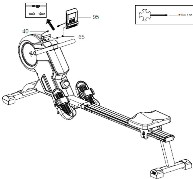
Remove the 2 Phillips screws (#65) that are pre-assembled on the back of the console (#95). Connect the sensor wires (#40) to the sensor wires on the back of the console (#95).
