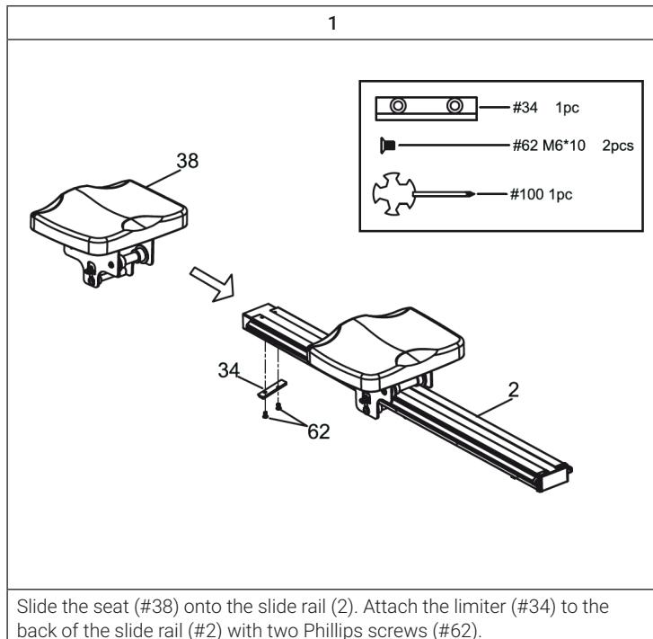
Slide the seat (#38) onto the slide rail (2). Attach the limiter (#34) to the back of the slide rail (#2) with two Phillips screws (#62).
