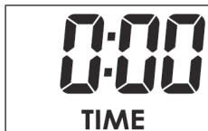
Press the UP or DOWN to set the desired time (1:00 to 99:00 minutes) and press MODE to confirm.
