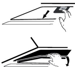
Two diagrams illustrating the removal of a filter. The top diagram shows a hand pressing a release button on a horizontal filter. The bottom diagram shows a hand pulling the filter out of its housing.                                              |
