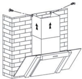
Insert the top chimney into the bottom chimney. Then pull the upper chimney out to the required height.
