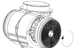
A diagram of a carbon filter being placed onto a circular fan or motor assembly. A curved arrow indicates the filter is being turned clockwise to align it with the fan's rotation.                                                                                      |
