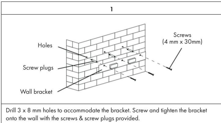
Drill 3 x 8 mm holes to accommodate the bracket. Screw and tighten the bracket onto the wall with the screws & screw plugs provided.
