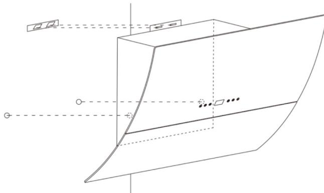
For inclined panel model, you need to drill 4 x 8 mm extra holes and use screw plugs and screws before installation.
