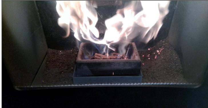
With correct combustion, as shown in the picture below, the ash container is practically empty. The flame (rich in oxygen) sparkles white and does not discolour the glass.
