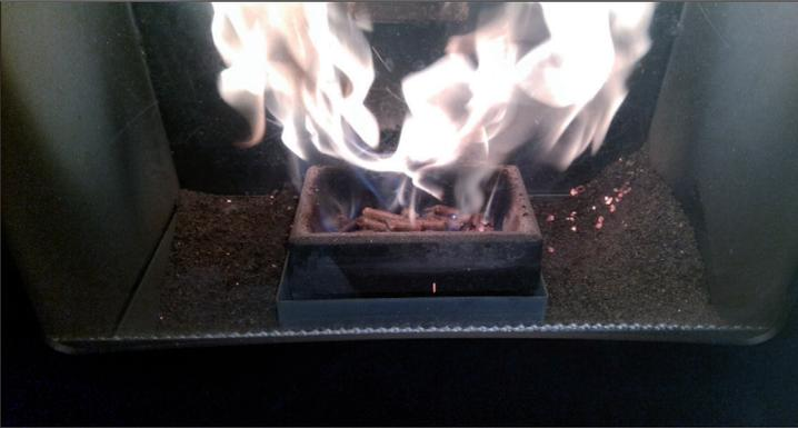
With correct combustion, as shown in the picture below, the ash container is practically empty. The flame (rich in oxygen) sparkles white and does not discolour the glass.
