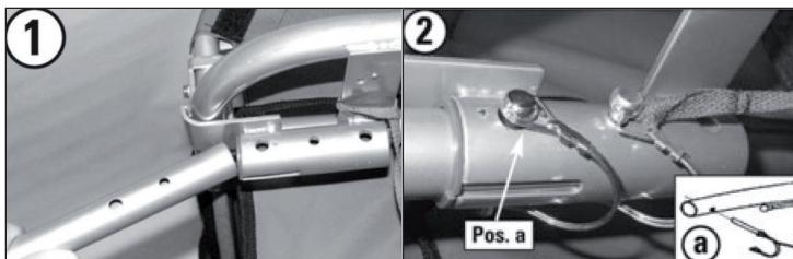
To attach the trailer hitch, slide the round end into the holder provided for this purpose (Fig. 1) on the left side. Secure the inserted drawbar with the supplied quick release (Pos. a) and the locking pin (Fig. 2). The curvature in the trailer coupling is now directed to the right in relation to the direction of travel.
