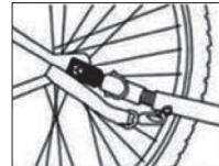
Secure the connection to the seat belt by wrapping it once around the bicycle frame (make sure it does not get into the spokes) and attaching it to the hanger part of the pull rod.
