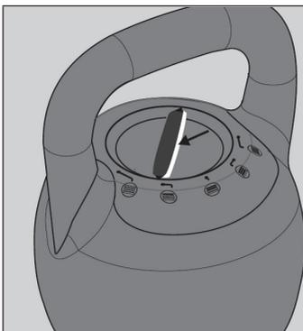
If the adjustment saucer is in the locking position, you should not be able to see the inner lever (yellow). If the inner lever is visible, adjust the outer lever slightly and the adjustment saucer will jump off.
