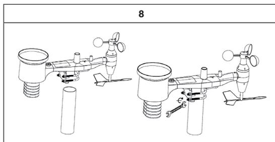
**Note:** Next to the antenna there is an arrow symbol with the inscription „WEST“ (see Figure 9), which represents the direction west. The device has been adapted so that the display shows „WEST“ in the direction of the real north. The use of a compass is recommended to determine the correct direction. A permanent wind direction error occurs when the outdoor sensor is not installed in the correct direction.
