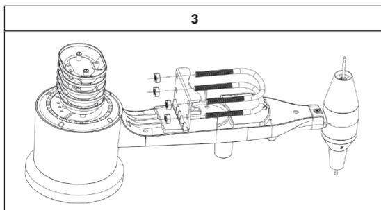
Loosely screw the nut onto the end of the U bolts. You can tighten the nuts after completing the installation (see Figure 4 for the final installation step).
