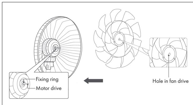
Remove the fan button from the packaging. Hold the fan blades with one hand and turn the fan knob counterclockwise with the other hand.
