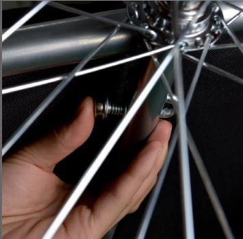
A close-up photograph showing a person's hands pulling a wheel off a hub. The wheel is detached from the hub, and the hands are shown gripping the wheel to remove it. <p>Para retirar la rueda, levante el remolque, pulse los botones del eje y retire la rueda (véase la ilustración).</p> |
