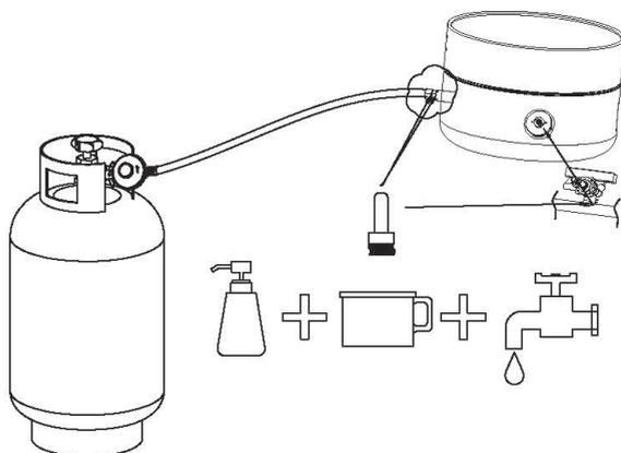
After the sealing glue has dried, close the valve and the gas supply completely. Use a soap solution to check for gas leaks. Apply soap solution to the connection between gas grill valve and connection.
