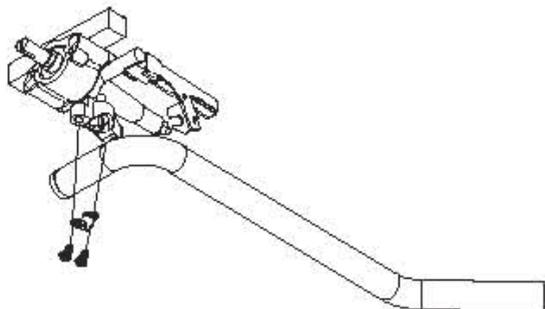
Attach the gas hose to the gas grill valve with a clamp and two screws (M5x12).
