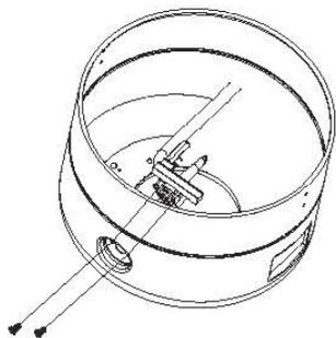
Mount the valve assembly to the controller using two screws (M4x8) and align the valve assembly so that the gas grill can be ignited using the rotary knob.
