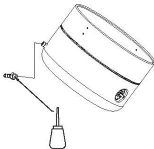
Apply some sealing glue to the connection thread and then attach the connection to the gas hose and tighten it.
