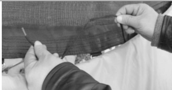
Use the string to connect the bottom of the safety net to the triangle rings as shown in the picture.
