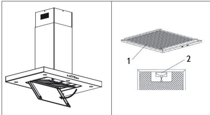
**Remove the filter as shown in the picture and then insert it again in reverse order.**
