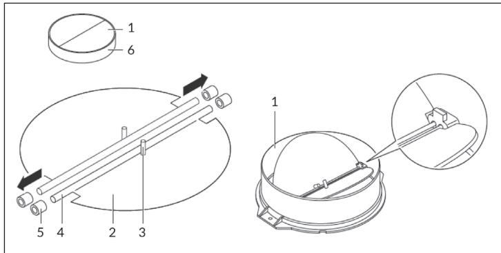
If you have an outside air outlet, the hood can be connected via a suction duct (enamel, aluminum, flexible tube or non-flammable material with an inside diameter of 150 mm) as shown on the right.
