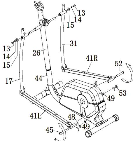
Fix the lower handlebars (17) and (31) to the upright post (26) with screws (13), washers (14) and D-shaped washer (15). Secure the pedal tubes (41L) and (41R) to the upright post (26) with the pedal joint bolts (45) and (52), spring washers (49) and nuts (48) and (53).
