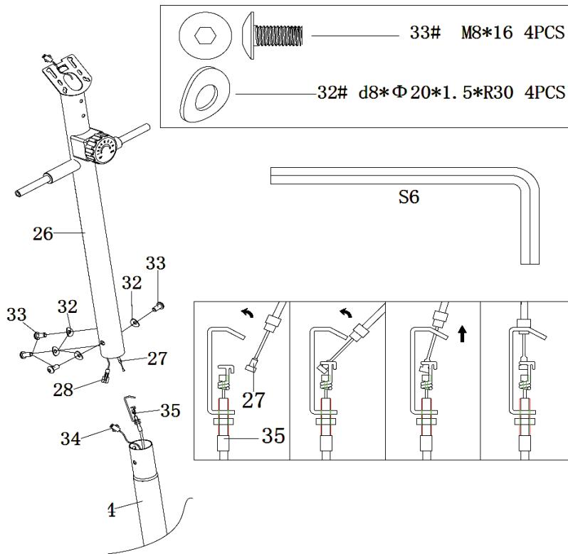
Connect the sensor cables (28) and (34), as well as the pull control wires (27) and (35). Fix the upright post (26) to the main frame (44) with screws (33) and washers (32).
