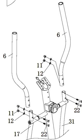
Attach the handles (6L) and (6R) to the lower handlebars (17) and (31) with screws (22), washers (12) and nuts (11).
