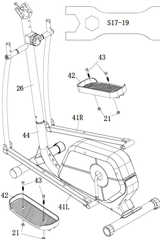
Secure the pedals (42) to the pedal tubes (41L) and (41R) with hexagonal bolts (43) and nuts (21).
