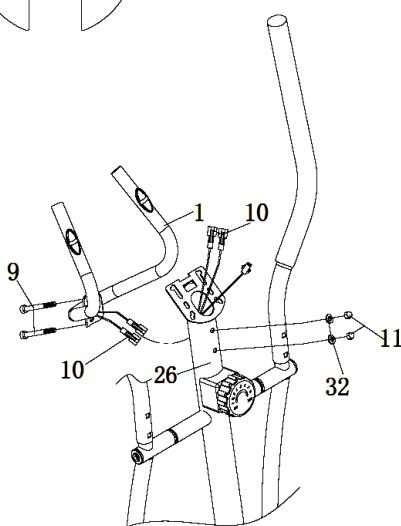
Connect the sensor cables (10). Secure the handlebars (1) to the upright post (26) with bolts (9), washers (32) and nuts (11).
