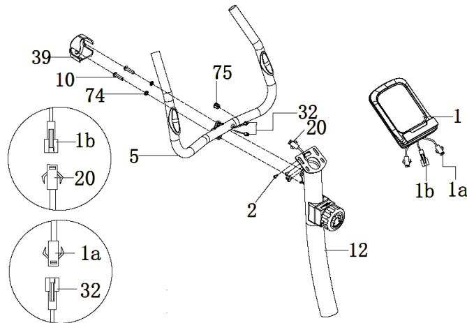
Fasten the handlebar (5) to the support tube (12) with a washer (74) and a screw (10). Connect the computer wire (1b) to the sensor cable (20). Connect the computer wire (1a) to the grip pulse wire (32). Fasten the console (1) to the support tube (12) with screws (2). Then attach the small cover (39) to the handlebar (5).
