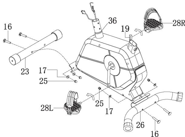
Attach the front anti-roll bar (23) and the rear anti-roll bar (26) to the main frame (36) with bolts (16), nuts (25) and washers (7). Attach the pedals (28L) and (28R) to the crank arms.
