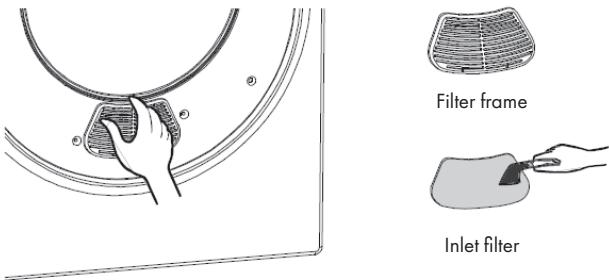
Clean the air inlet filter once a month. Remove the filter by holding the lower and upper ends of the frame and pulling it out. Clean the inlet filter with a soft brush. Then replace the filter in the frame and secure the frame.
