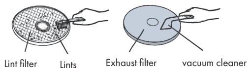
Separate the filters. Clean the filter cover, lint filter and exhaust filter with a soft brush or vacuum cleaner. Be careful not to damage the filters.
