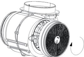
A detailed diagram of a circular duct assembly. An activated carbon filter is shown being inserted into a flange on the side of a larger duct. A curved arrow indicates the insertion path of the filter.                                                |
