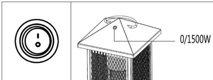
First switch the device on at the on/off switch (left picture). Then press the touch switch (right picture) once to operate the heater with 1500 W. Press the touch switch a second time to switch off the heater.
