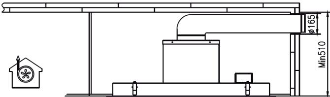
You can either discharge the exhaust air to the outside or operate the extractor hood in recirculation mode (upper pictures). If you discharge the air, attach the end of the exhaust pipe to the outlet in your ceiling or wall (bottom picture).
